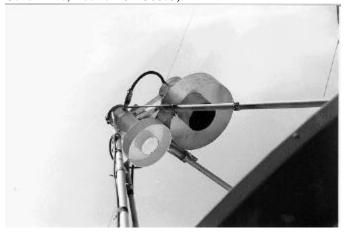
Note also how dual feedhorns can be accommodated by mounting one horn slightly offset from the focal point of the dish. This approach skews the antenna pattern slightly, but the result is easily measured by peaking the antenna on sun noise, and compensating aiming accordingly. Such a dual feedhorn design is a viable alternative for those members wishing to use a single dish simultaneously for satellite TV reception and SETI.
