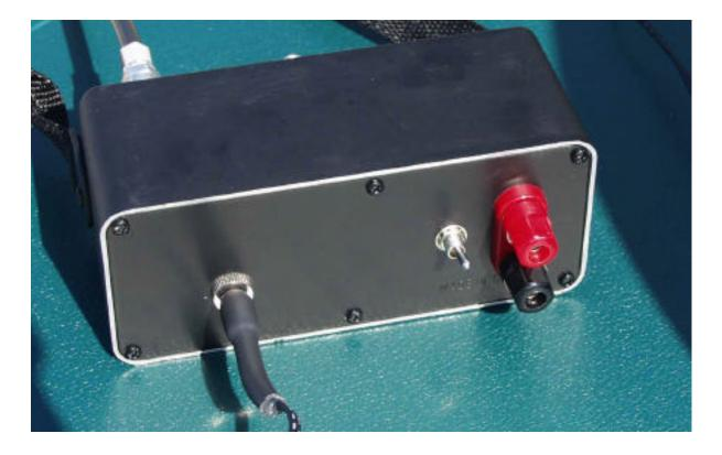
In the above photo you can see where I input the 12-15 vdc and output the voltage from the meter to the recording device. The toggle switch connects the output to either the meter or a 10,000 ohm resistor. The binding posts make the output across the resistor available for logging.
