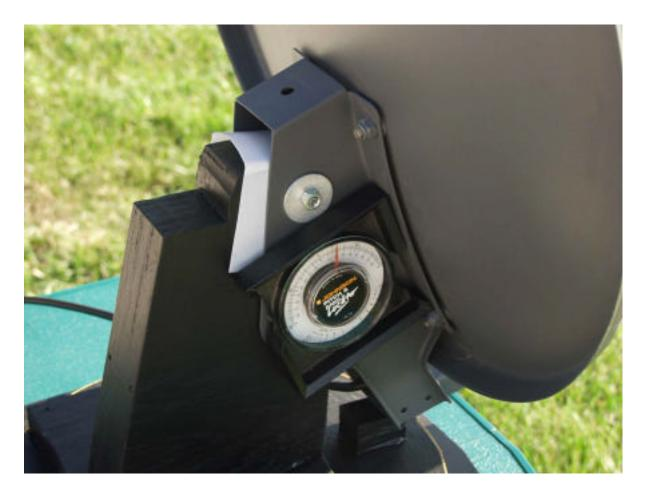
The readout will not be accurate, but the experiment below will help you determine the correction factor. Hot plastic glue holds the protractor to the dish just fine.
