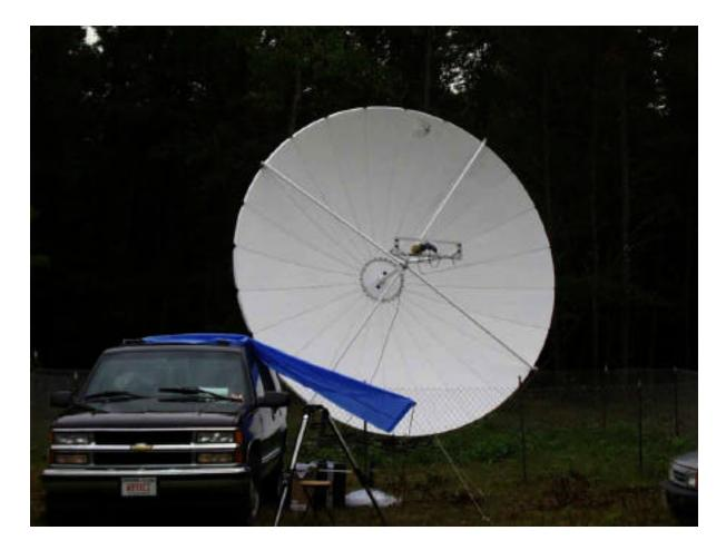
In order to spur a little more interest I introduced the LBT2, a 12,000 MHz radio astronomy telescope you can build for less than \$200. Here two star party members, Jacki Lavaque and Daniel Blomquist experiment with the neat little radio telescope:
