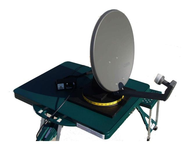
A simple RF/IF/Detector unit is a Channel Master Model 1004IFD tuning meter that includes an **audible tuning indicator**.
