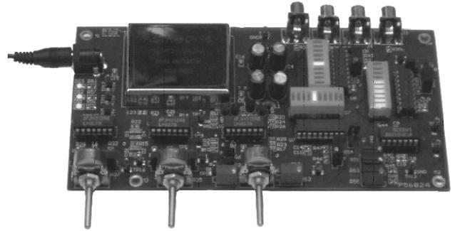
Fig. 8. Analog test fixture for limited frequency tuning and beam steering.
