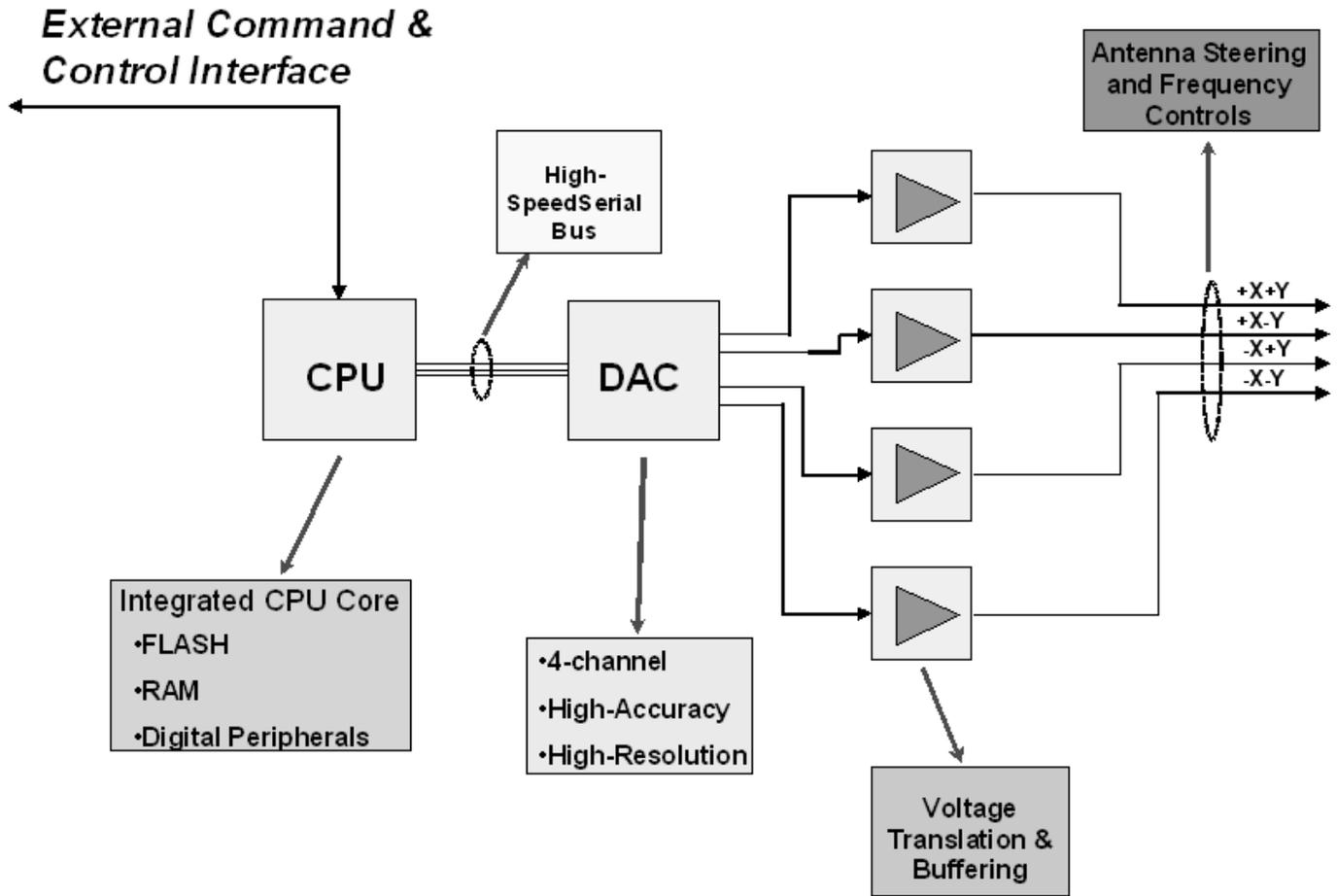
Fig. 5. Mission-specific digital control circuitry.
