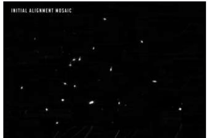
This mosaic image shows the alignment process of the JWST's segmented mirror. According to NASA's February 2022 blog post, this image helps to "confirm that NIRCam was ready to collect light from celestial objects, and then identify starlight from the same star in each of the 18 primary mirror segments. The result is an image mosaic of 18 randomly organized dots of starlight, the product of Webb's unaligned mirror segments all reflecting light from the same star back at Webb's secondary mirror and into NIRCam's detectors. What looks like a simple image of blurry starlight now becomes the foundation to align and focus the telescope in order for Webb to deliver unprecedented views of the universe this summer. Over the next month or so, the team will gradually adjust the mirror segments until the 18 images become a single star."
