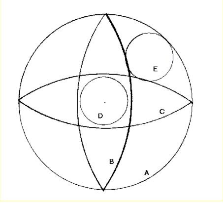
Figure 2 Beam Pattern, plotted in Elevation vs. Azimuth, of the Adaptive Microwave Array in its five operating modes.
