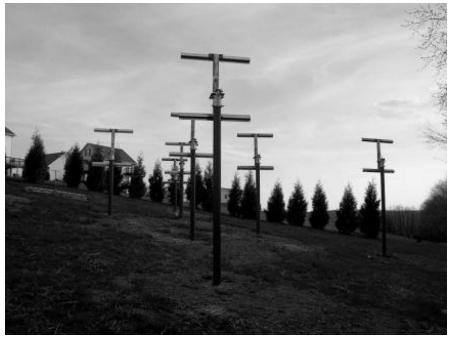
Figure 13 Azimuth-Elevation mounts installed on the remaining VSA masts, awaiting arrival of their dishes.
