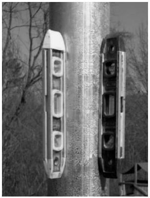
Figure 7 Two magnetic bubble levels, attached at right angles, facilitate leveling the masts.
