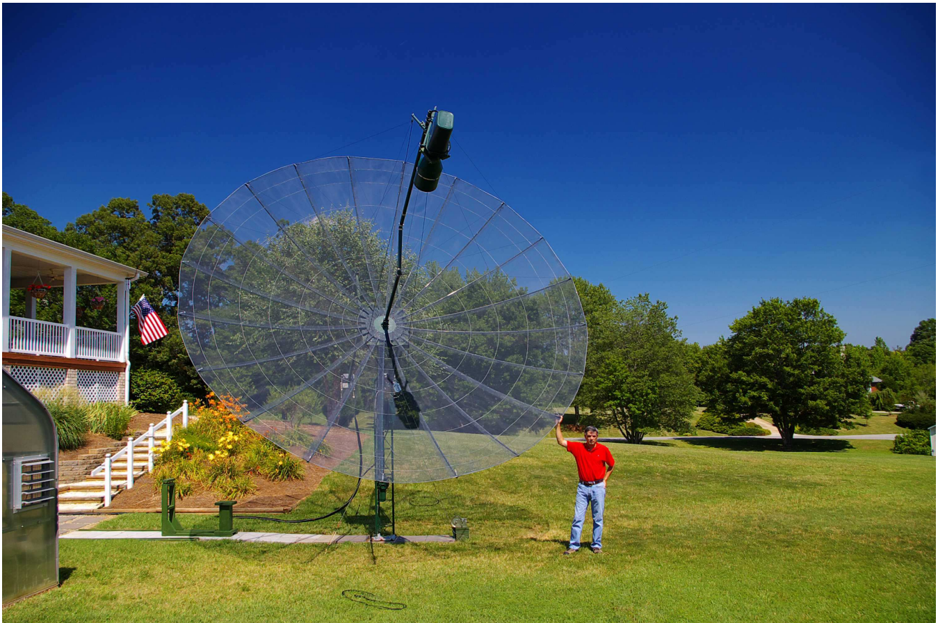
SETI League member Marc Franco with his newly constructed 20 foot diameter stressed parabolic dish antenna in North Carolina, USA. (N2UO photo)
